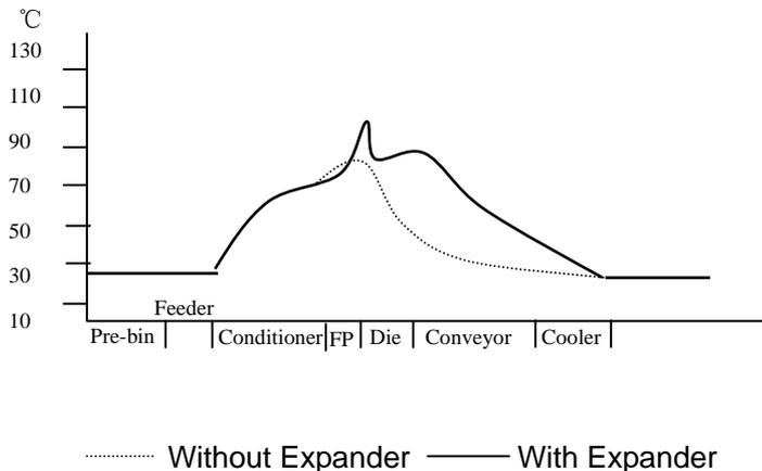
Fig.1 Feed temperature in typical expanding process
