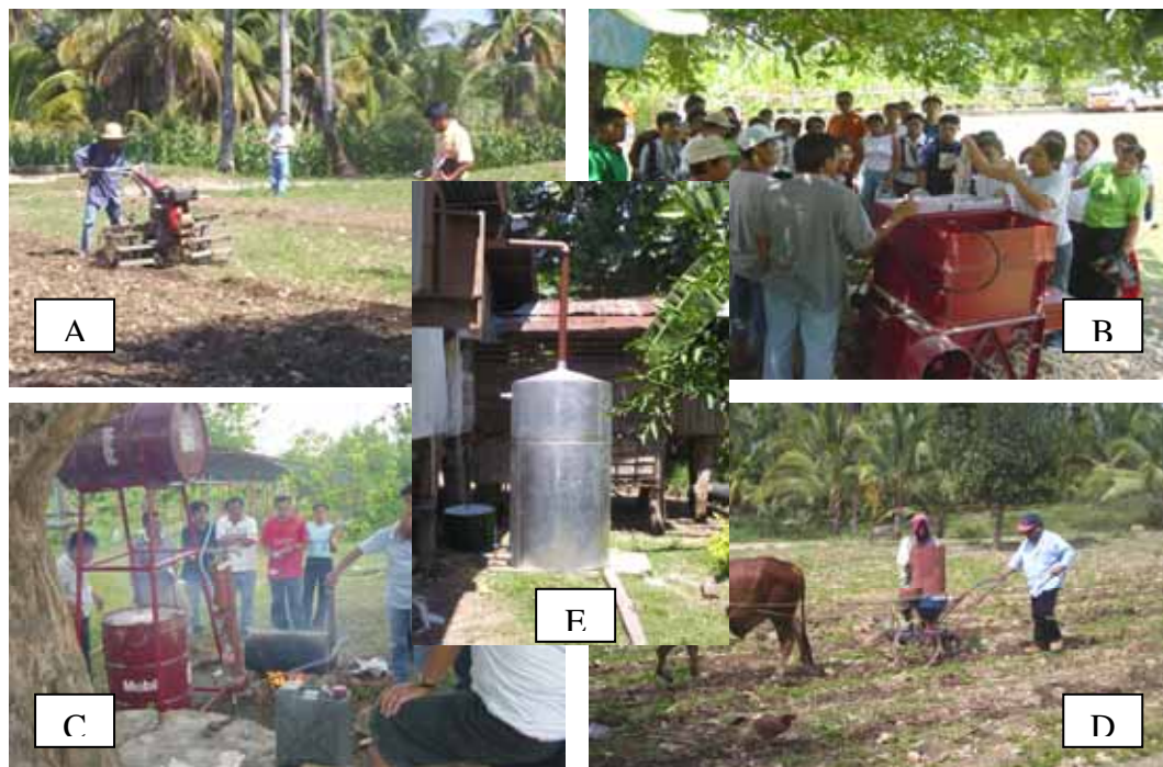
Figure 3-16. Machines and equipment brought to the pilot site in Tongo, Argao, Cebu as part of the introduction of corn mechanization technologies in the pilot farm: (a) power tiller, (b) corn sheller, (c) ethanol extraction system, (d) organic fertilizer applicator, and (e) collector for rain harvesting system.
