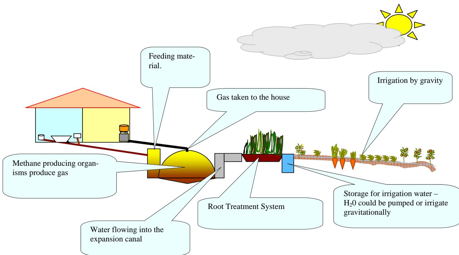
**Sketch of biodigester replacing a septic tank.** Wastewater as well as kitchen and garden waste enter the digester and are broken down to biogas and fertile water.
